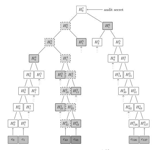
Fig. 1: The figure represents the Merkle tree for a chunk  $(H_i^{\lambda} \stackrel{\text{def}}{=} \mathcal{M}_{2,\mathcal{H}}(c,\lambda,i))$ . Shaded in grey in the middle is the Merkle proof for index 42 (7-bit binary representation is 0011010). The proof can be verified knowing only the data segments at the given index j = 42 and its sister segment (next segment if index is even, previous if odd), plus sister hashes at each level as indicated.
