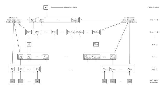
Fig. 4: The swarm hash construct. Hierarchical chunking.
