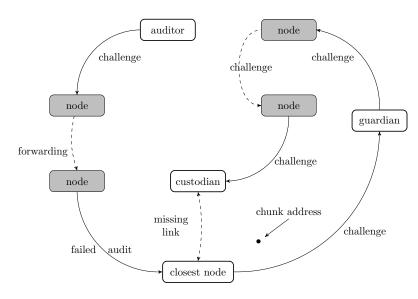
Fig. 6: The arrows represent local transactions between connected peers. After the audit reaches the closest node and the chunk is not found, the closest node challenges the guardian who in turn challenges the node it originally bought a receipt from, and so on until the challenge lands on the current custodian who now has the chance to connect to the node that is actually closest to the chunk address (or at least closer).
