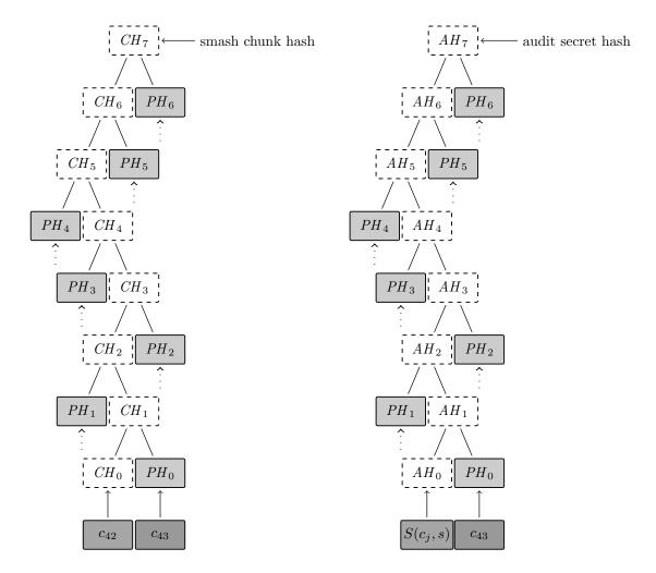
Fig. 2: Given a chunk hash, a seed, and the index, the audit secret hash for ASH(c, s, j) can be calculated and verified using only the Merkle proof for the segment at the index. The left hand side is the Merkle structure of the original segmented chunk, the right hand side represents the corresponding Merkle proof for the audit secret.
